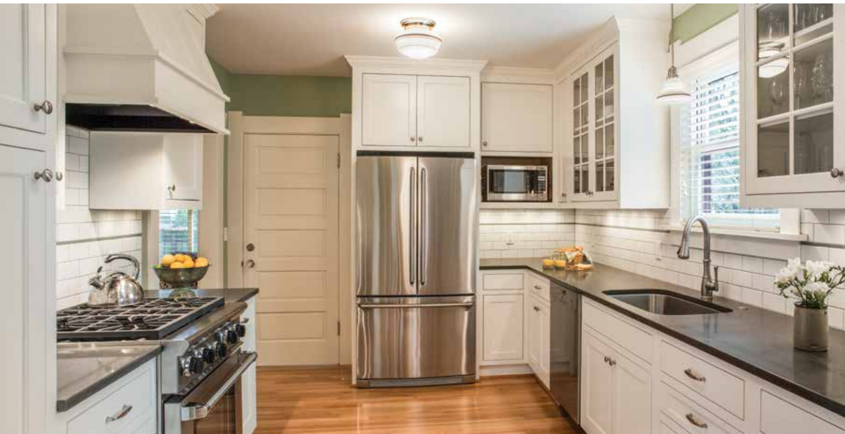
ABOVE Custom and period touches include locally made, raised-panel cabinetry flush-mounted to the ceiling and a subway-tile backsplash with accent strip coordinated to the wall color. The counters are Cambrian granite with a texturized surface, a finish process similar to honing, done by wire brushing. LEFT Relocating the refrigerator made space for a broad entry passage to the new sitting room.
